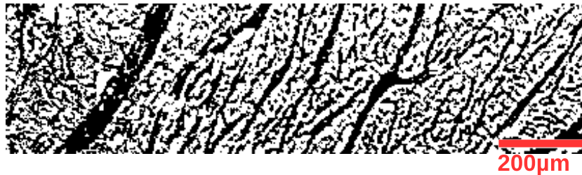
Fig. 4: Binary thresholding of Fig. 3c with a manually-chosen threshold.
